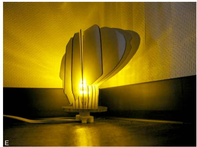
Figure 8. Creating a lamp shade with Spatial Sketch , (A) The original 3D sketch (B) Radial slices of the sketch (C) Laser cut slices of card, (D) The final set of parts before assembly, (E) The final assembled lamp shade.
